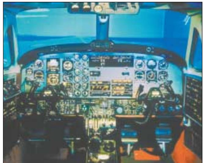
Microprocessors have replaced conventional hydraulic motion platforms in the Pan Am SimCom flight simulator for the Beechcraft King Air B-200. Separate electronic systems recreate the visual, motion and sound experiences critical to pilot training.
