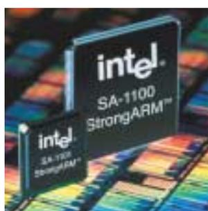
f. StrongARM chip: printing, scanning, portable computing
