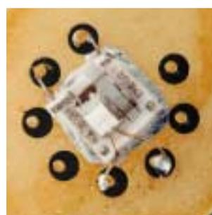
h. Hygrometer chip: measuring moisture
